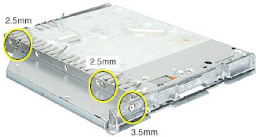
7. Remove the bottom L-shaped EMI bracket.
