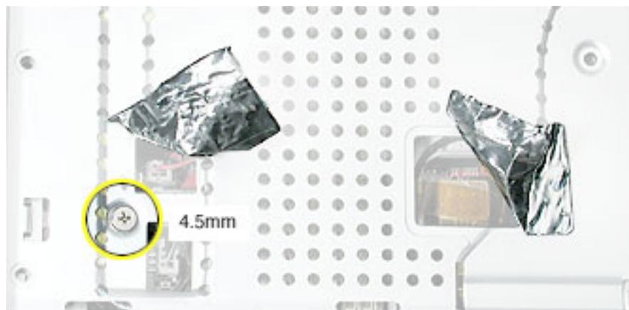
6. Remove two screws from the front right side of the top case.
