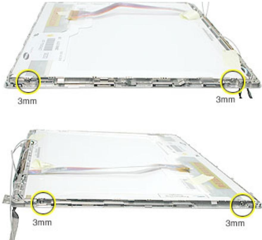
3. Lift off the long EMI clip at the base of the bezel.
