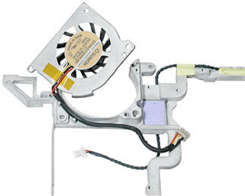
3. Secure the replacement fan to the frame, and reassemble and test the computer.
