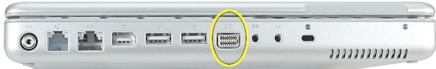
The mini-DVI port is used with an adapter cable to connect the computer to a monitor, television, VCR, or other video device. The adapter cables that can be used with this port include a mini-DVI-to-DVI adapter, a mini-DVI-to-VGA adapter, and a mini-DVI-to-S-Video adapter.
