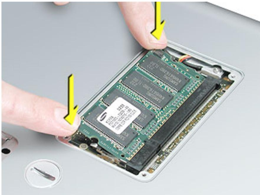
8. Install the memory door. Be careful not to overtighten the screws.
